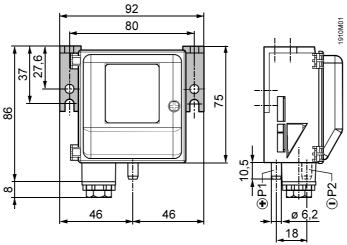
Air duct probe (ABS)
