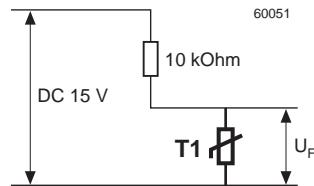
This circuit produces a change in voltage of 10 mV for each 1 K temperature change. There is a directly linear relationship between the sensor voltage  $U_F$  and the temperature across the entire sensor measuring range.
