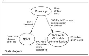
In the Power-up state, the green LED blinks "Off-line". The device is open for *both* SNVT and TAC Xenta I/O module communication.
